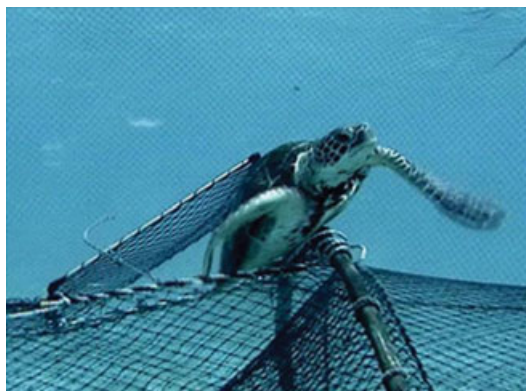
Figure 7 Turtle releasing device tested in the small-scale Japanese pound net fishery. The fishery employs cone-shaped traps, which are relatively small, have a circular cross section and have relatively stable net tension. The high tension causes the device's flap to automatically close, where turtles can open it but not fish (Abe and Shiode 2009).
